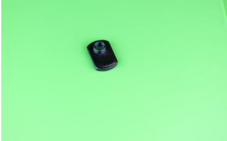
Fig. 4. The image of a test sample is shown above. The object is automatically detected in the image. Effective object detection depends on appropriate lighting and background. Numerous images, taken from various elevation and azimuth angles, are then reconstructed into a 3D representation using a space carving algorithm.
