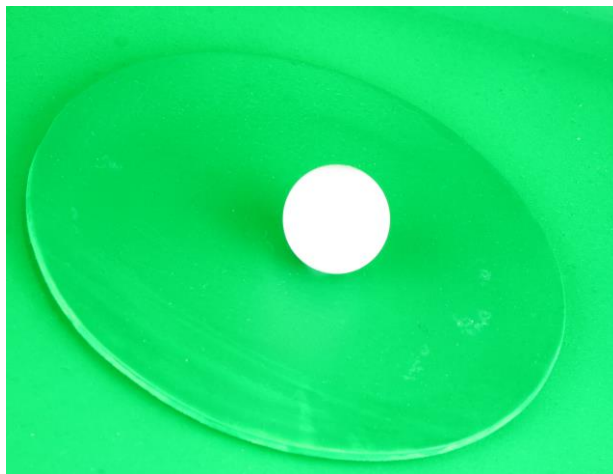
Fig. 7. The calibration sphere shown above is used to ensure accuracy of the imaging system measurements. The sphere, which has a known diameter, is imaged after calibration to ensure that the measurement is within the required accuracy threshold.
