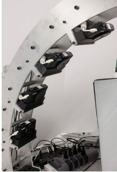
Fig. 2. Four of the point-and-shoot digital cameras used in the system are shown above. They are rigidly mounted to the support structure. The white cable connected to each camera allows for computer automation of image acquisition. To eliminate the need for recharging the cameras, the battery in each camera has been replaced with an external power source.
