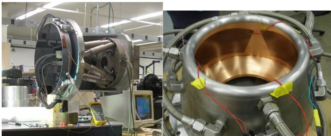
Fig. 7 Left: Tip/Tilt secondary mirror. Right: Prime focus heat stop.
