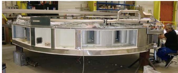
Fig. 6 Left: The University of Arizona Optics lab showing (from front to back) the polishing support rig, stressed lap polishing head, the M1 blank in its box, and a commissioning blank (also produced by SCHOTT-AG) at the back of the room. Right: M1 cell assembly at AMOS in Begium.
