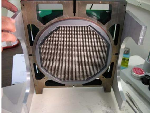
Fig. 8 The deformable mirror actuator array during assembly at Xinetics.
