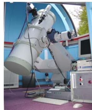
Fig.2(b). Fork-type mount and 35cm telescope
