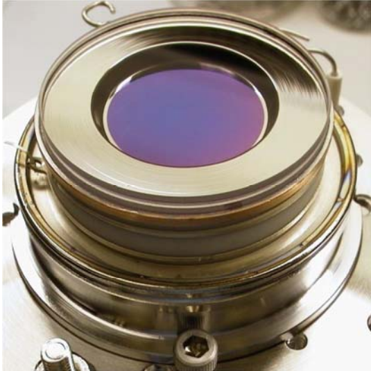
Fig. 1. 25 mm cross delay line anode, MCP, sealed tube with S20 photocathode.
