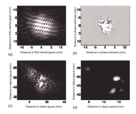
Figure 4: Results of compressive sensing reconstruction of three LEDs aberrated by turbulence. (a) The reconstructed coherence function of the LEDs without turbulence. (b) The estimated phase of the aberration. (c) The image neglecting turbulence, showing the distortion produced by turbulence. (d) The estimate of the source intensity without turbulence.
