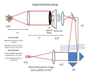
Figure 3: Diagram of the setup to measure the cross-spectral density from LEDs with a phase distortion.
