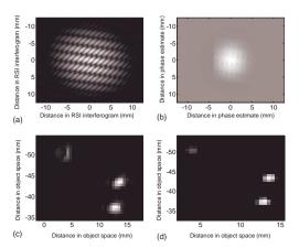
Figure 5: Results of a control experiment of compressive sensing reconstruction of three LEDs not aberrated by turbulence. (a) The reconstructed coherence function of the LEDs. (b) The estimated phase of the aberration, which is close to null because no turbulence is present. (c) The image of the original source. (d) The estimate of the source intensity, which improves the image quality because the L1 constraint sharpens the points slightly.
