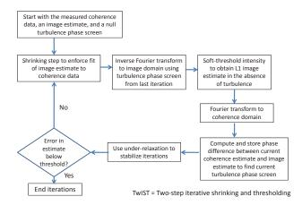
Figure 2: A block diagram of the compressive sensing algorithm used to find the unaberrated image and a turbulence estimate.
