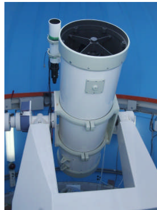
Fig. 2. 35cm Telescope and 2K2KCCD camera
