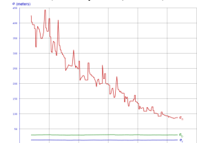
Figure 5. The RMS of the errors of determination of the position of Kosmos-2251 spacecraft for the time of collision with Iridium-33 spacecraft.
