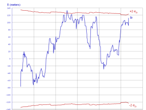
Figure 13. The real and calculated ( 2\sigma ) errors of determination of relative position of Kosmos-2251 and Iridium-33 spacecraft for the time of collision for \sigma_r (numerical prediction, field 8x8, no adaptation).
