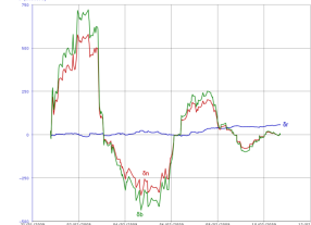
Figure 2. The errors of determination of relative position of Kosmos-2251 and Iridium-33 spacecraft for the time of collision (numerical prediction, field 8x8).
