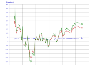
Figure 4. The errors of determination of relative position of Kosmos-2251 and Iridium-33 spacecraft for the time of collision (numerical prediction, field 36x36).
