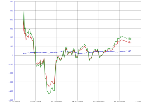
Figure 3. The errors of determination of relative position of Kosmos-2251 and Iridium-33 spacecraft for the time of collision (numerical prediction, field 16x16).
