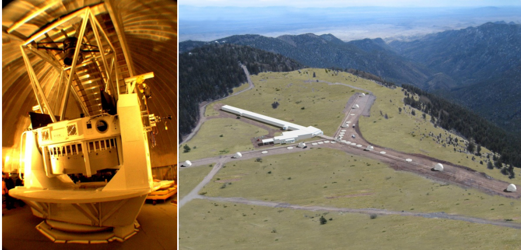
Figure 1. Two telescope facilities atop Magdalena Ridge. On the left is the fast-tracking 2.4m telescope which is now in operations. On the right is our architect's conception of the MROI facilities. The equilateral Y configuration with 28 pads is clearly visible to the right of the interferometric buildings.
