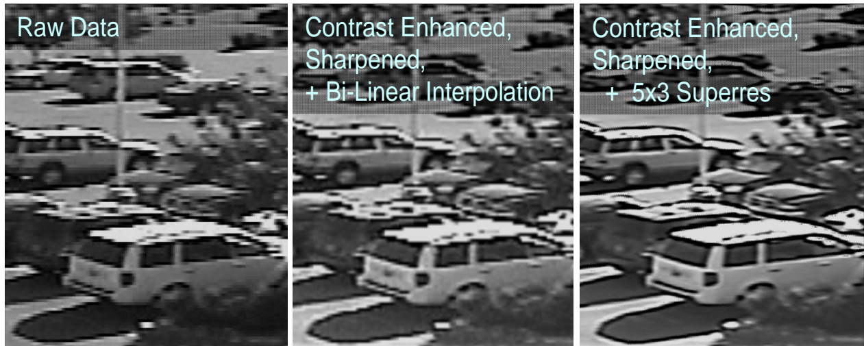
Fig. 4. Application of SRTIE to video data captured with a home consumer grade video camera. The middle panel shows the image resulting from 3x upsampled bilinear interpolation of the raw image, which compared to the SRTIE processed output in the right-hand panel clearly shows SRTIE has achieved a strong degree of superresolution.
