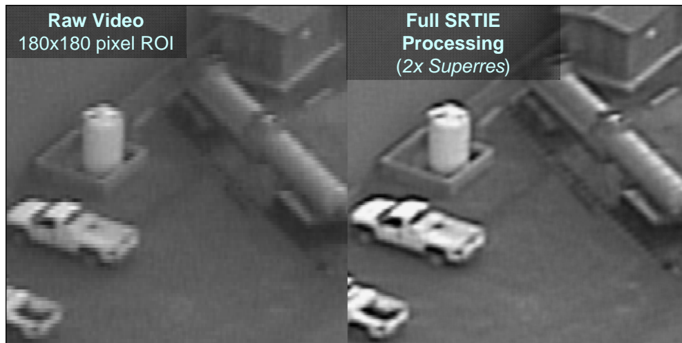
Fig. 5. Application of SRTIE to a live video feed from a visible band camera hosted on a Scan Eagle unmanned air vehicle.
