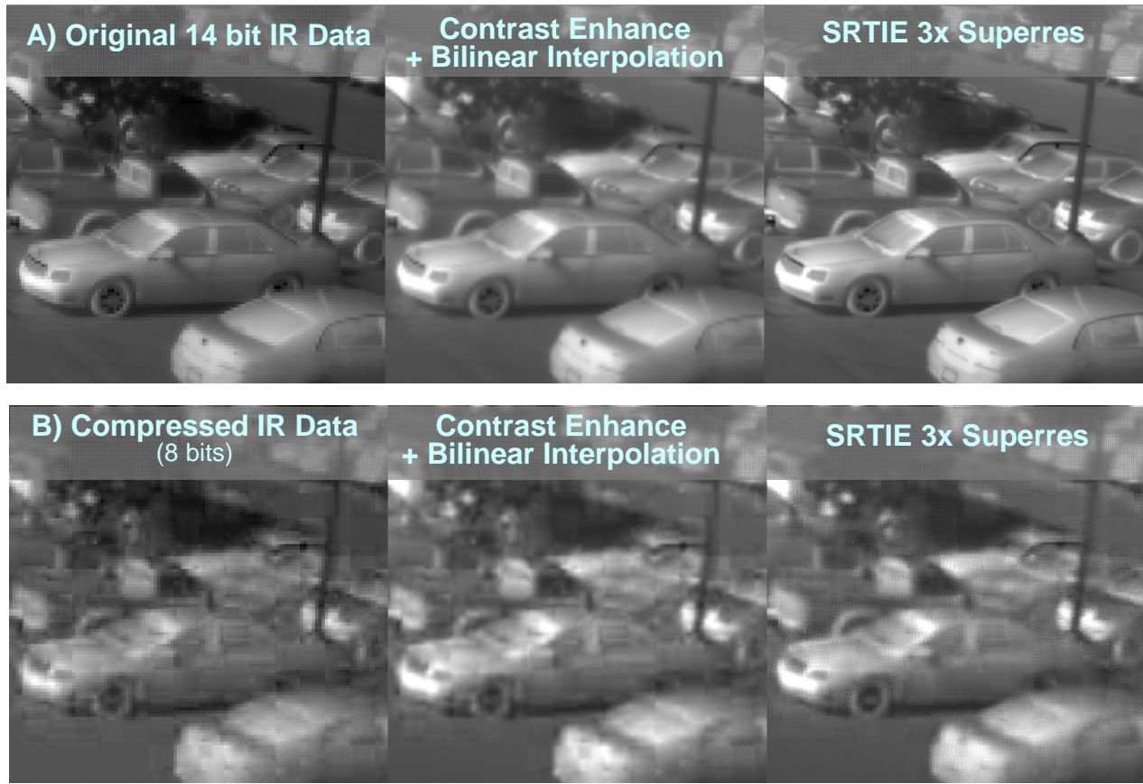
Fig. 6. Application of SRTIE to video data captured with a 14 bit IR camera. The upper row (A) shows processing of the original raw data, while the lower row (B) shows processing of the IR data after MPEG compression. The upper row shows clear evidence of superresolution. SRTIE processing of compressed data is not able to recover the original quality but does strongly suppress compression artifacts.
