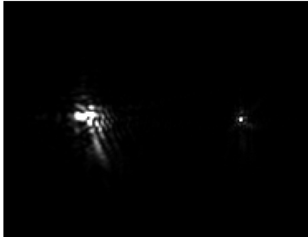
Fig. 5: An image of an aberrated beam before and after correction using the holographic wavefront sensor and MEMS mirror.
