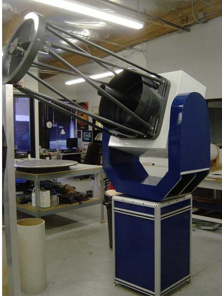
Figure 3- Lightweight telescope mounted on portable AO system and lightweight mount.
