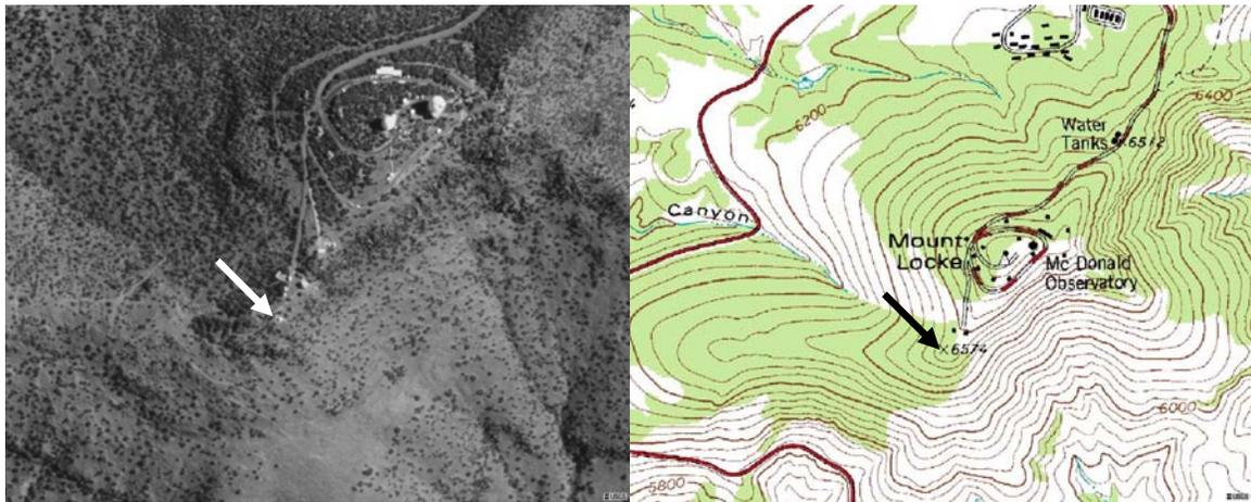
Fig. 2. The CTI-II site on the southwest ridgeline of Mt. Locke. The site is favorably located into the prevailing winds and takes advantage of relative orographic isolation both from topology and from other buildings and structures.
