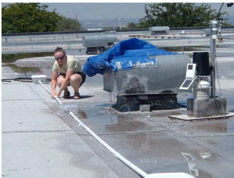
Fig. 9. UNM graduate student M. Suzanne Taylor tests a microbarograph array element. The differential atmospheric pressure between the two open ends of the 10 m element is measured by a sensitive differential pressure sensor in the middle box immediately in front of Suzanne. Each end of the element has baffling to preclude saturating the sensor on wind-induced noise. The pressure sensor is read at a 10Hz rate under control of LabVIEW.
