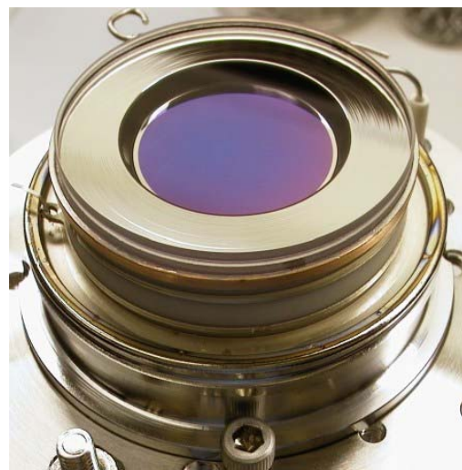
Fig. 10. 25mm sealed tube cross delay line detector.
