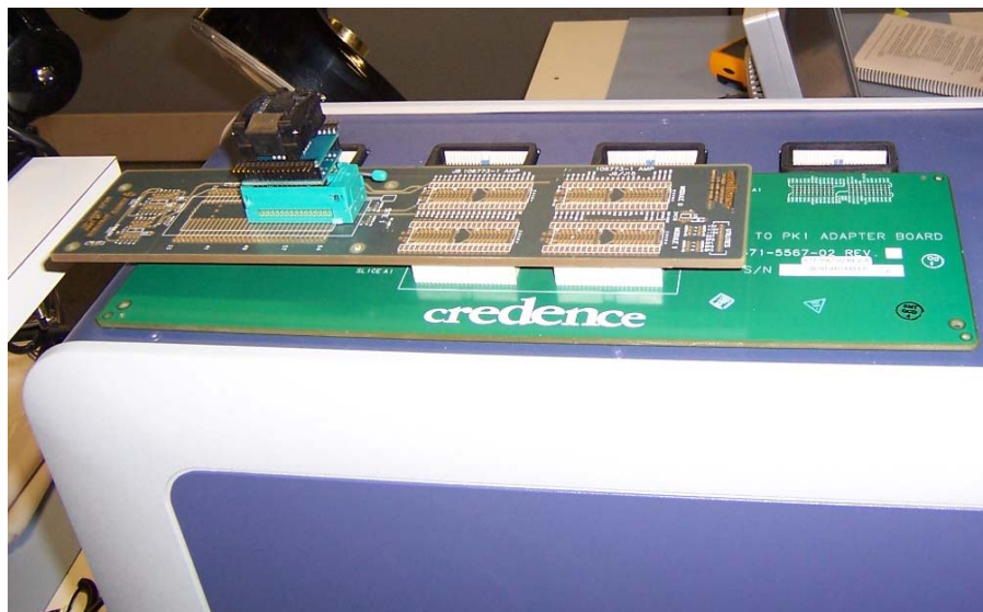
Figure 3: Top view of the Credence PKII with a memory chip test board attached.
