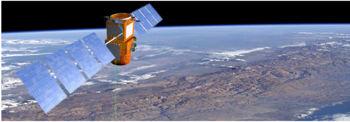
Figure 4: Artistic impression of the CALIPSO (Cloud-Aerosol Lidar and Infrared Pathfinder) Satellite, for atmospheric observations [10]. CALIPSO was launched on April 28, 2006, and is presently in a polar orbit, in formation with five other atmospheric satellites, at 705 km altitude. CALIPSO contains a Nd:YAG laser, producing light at 523 nm and 1064 nm wavelengths, which can accurately point at a given location on the globe. We plan to take test data at Palomar Observatory later this year with light pulses from the CALIPSO laser.
