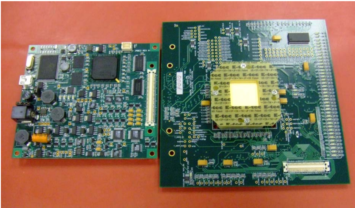
Figure 9: Ambient temperature ASIC board and JADE-2 interface board.
